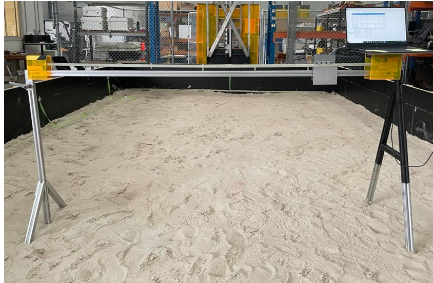
Figure 6-4. Pin profiler for surface roughness measurements.
