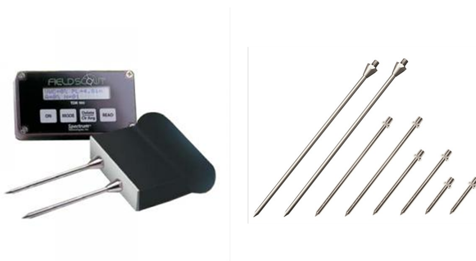
Figure 5-6. Scout Sensor and pins (sizes of pins for this study: 3.8cm (1.5in), 7.6cm (3in), 12cm (4.7in) and 20cm (7.9in))
