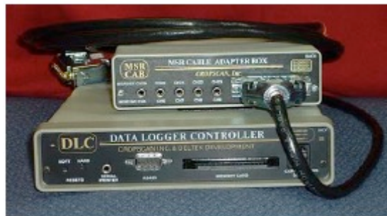
Figure D-2. Data logger controller & cable adapter box.
