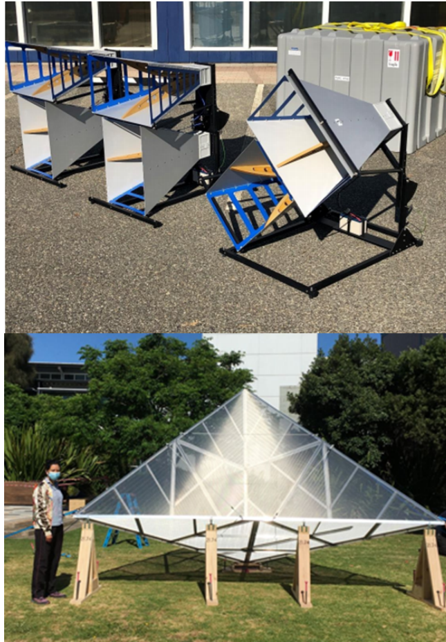
Figure 4-6. Polarimetric Active Radar Calibrators (top) and Passive Radar Calibrator (bottom).
