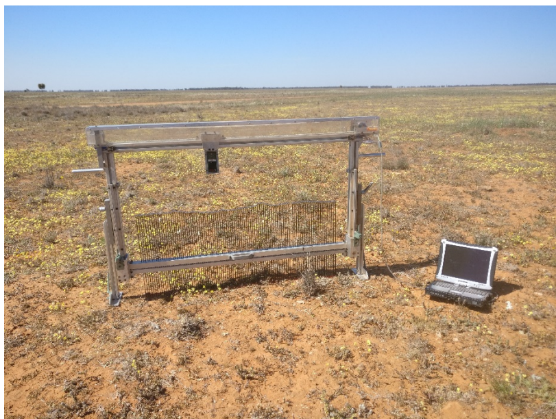
Figure 6-5. Laser-pin profiler for surface roughness measurements.
