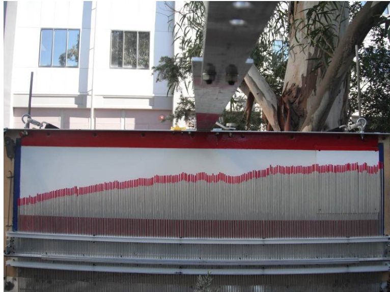
Figure 6-3. Pin profiler for surface roughness measurements.
