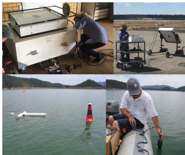
Figure 4-4. Upper right: undertaking a sky cold point calibration; upper left: undertaking a warm point calibration with the calibration box shown in the inset; lower left: the buoy used to monitor water temperature and salinity; lower right: undertaking a boat transect of water salinity and temperature.
