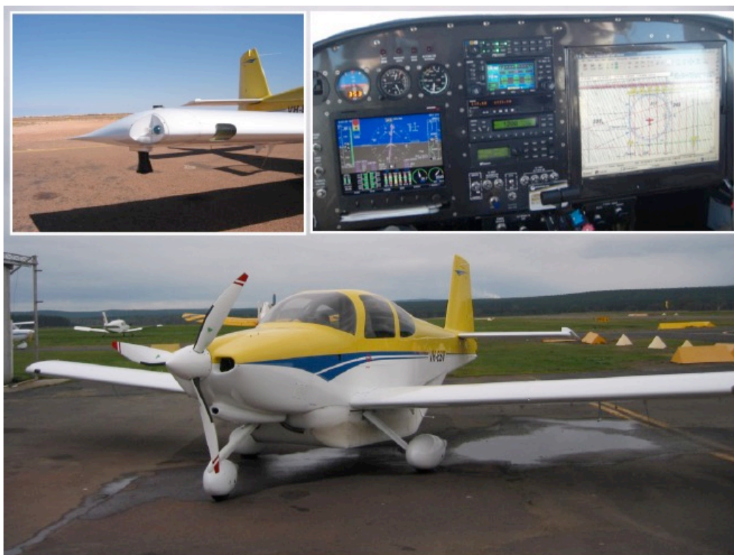
Figure 2-1. Experimental aircraft showing a wingtip installation in the left inset, and the cockpit with cockpit computer display in the right inset.
